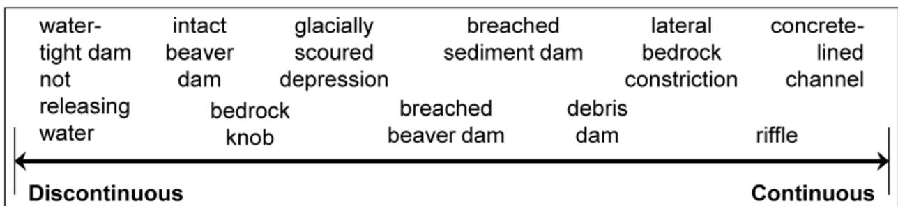
**Figure 4.** Examples of features along a river corridor on a gradient from discontinuous to continuous, where the entirely continuous feature allows all water and sediment to flow through the cross section unmodified, and the discontinuous feature blocks all water and sediment flow. Each of the feature types provided here as an example has a range along this gradient depending on factors such as the size, materials, and condition of the feature.
