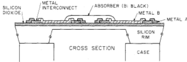
Figure 7 – A monolithic silicon thermopile detector fabricated using integrated circuit technology (Lahiji & Wise 1982, Figure 1)
