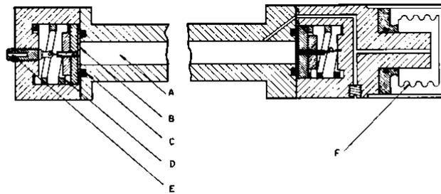
Figure 2- Schematic of NOL’s velocimeter; similar to the velocimeter used by NBS (Wilson 1959, Figure 1)
