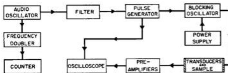
Figure 3- A block diagram of the instrumentation used by NOL for the electronic component of their double-crystal velocimeter (Wilson 1959, Figure 2)
