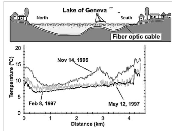
Figure 8 – Temperature transects taken between France (south) and Switzerland (north) using existing communication fibers under Lake Geneva (Selker et. al 2006, Figure 2)
