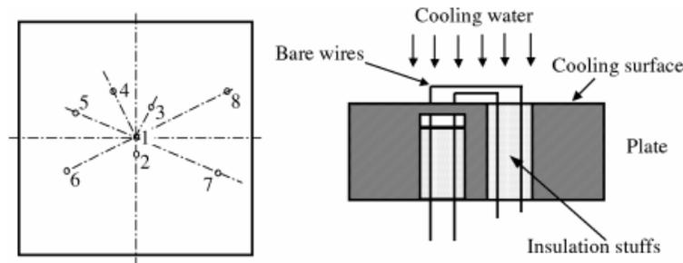
Figure 6 - Schematic installation of TC's used by Xu & Gadala (Xu & Gadala 2005, Figure 3)
