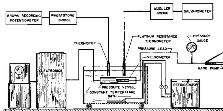
Figure 4- Diagram of the general arrangement of the instrumentation used by the Naval Ordnance Laboratory (Wilson 1959, Figure 3)
