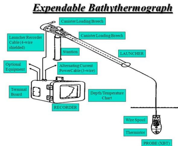
Figure 1- Diagram of an expendable bathythermograph (Speed of Sound in the Sea 2018, Figure 3)
