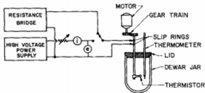
Figure 5 - Apparatus employed to determine the velocity dependence of the dissipation factor (Rasmussen 1962, Figure 1)
