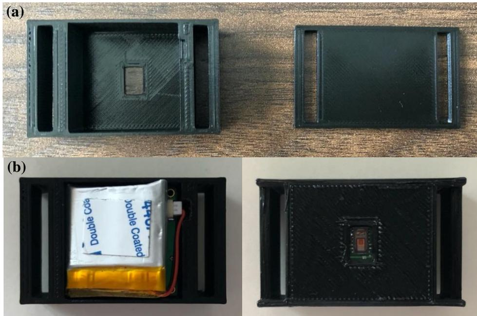
*Figure 3. Final and optimal design of enclosure (a) without sensor and (b) with sensor.*
