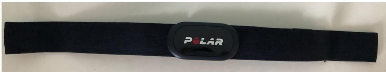
*Figure 6. Polar H10 sensor incorporated in a chest strap.*
