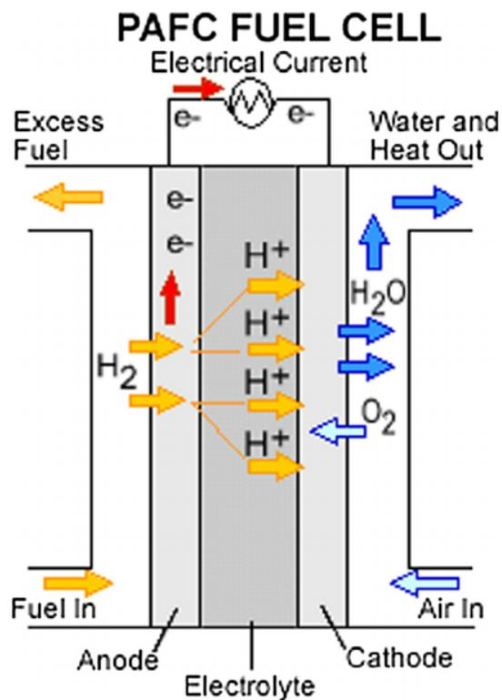
Figure 1: Schematic of Phosphoric Acid Fuel Cell (PAFC) [3]
