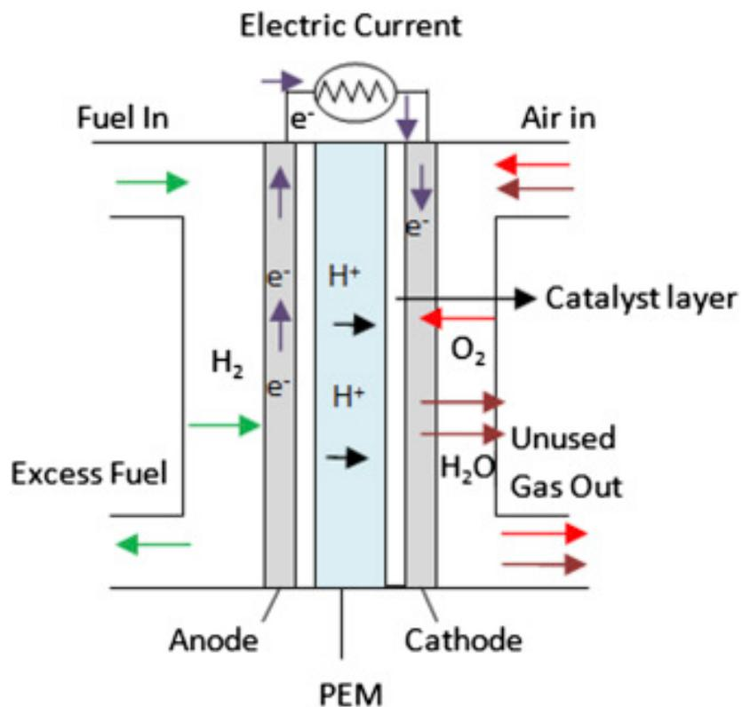
Figure 2: Schematic of Proton Exchange Membrane Fuel Cell (PEMFC) [4]
