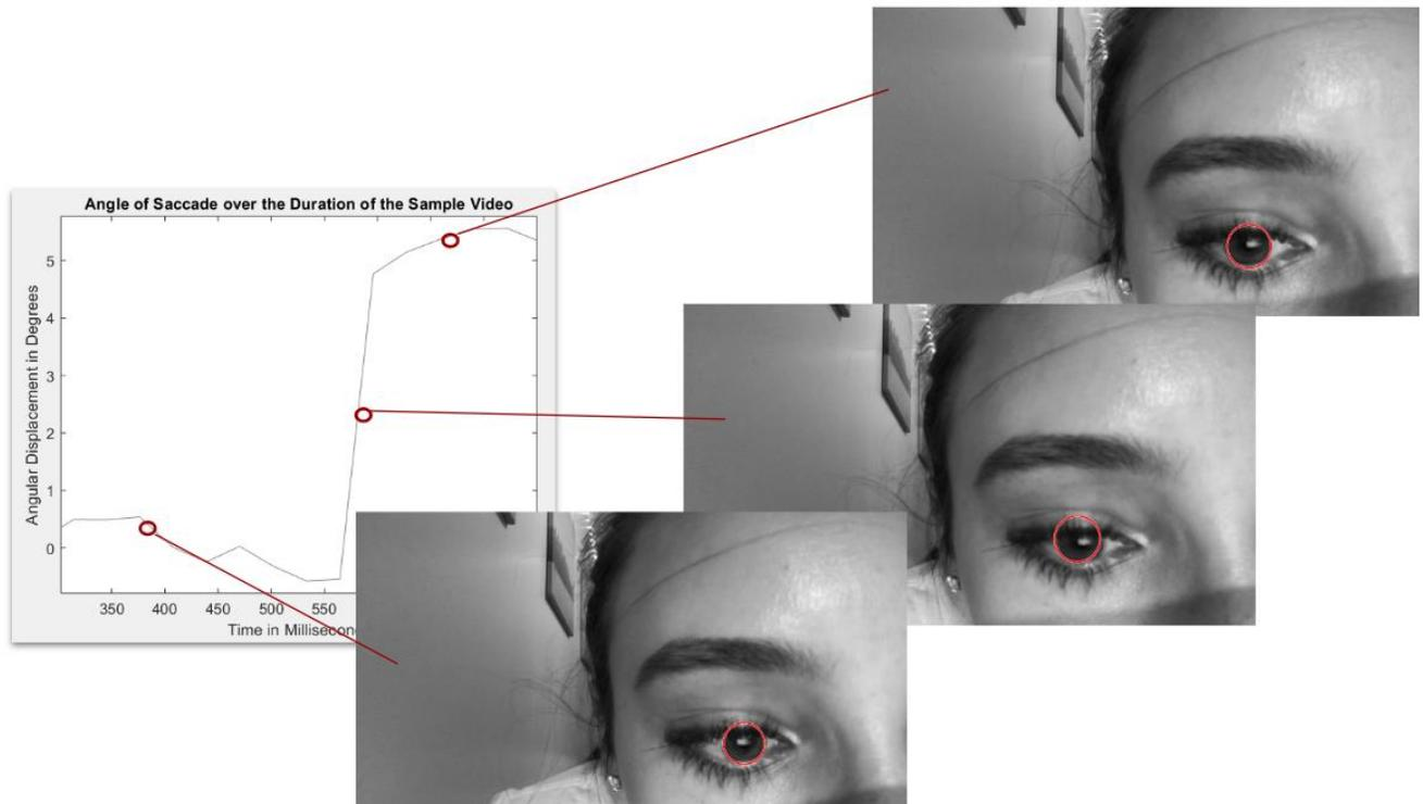
**Figure 24 Saccade plot from final software setup and preliminary hardware design shown correlated with individual frame iris detection over saccade duration**
