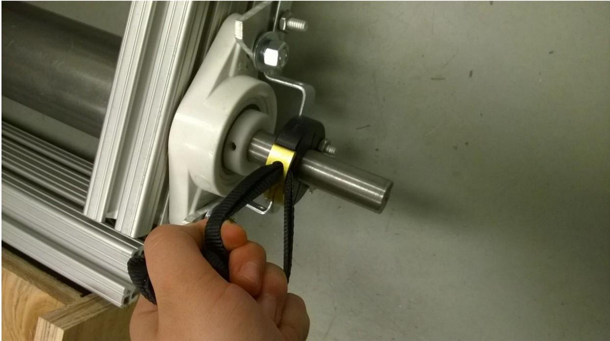
**Image 3: Closeup of brake with fabric handle**
