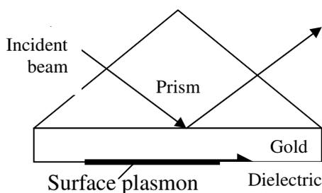
Figure 1. Kretschmann prism configuration [3]
