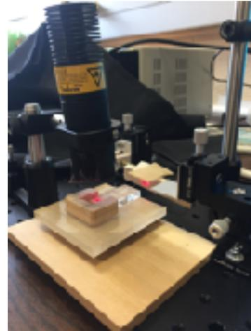
*Figure 1. Wooden platform aligning optical components.*
