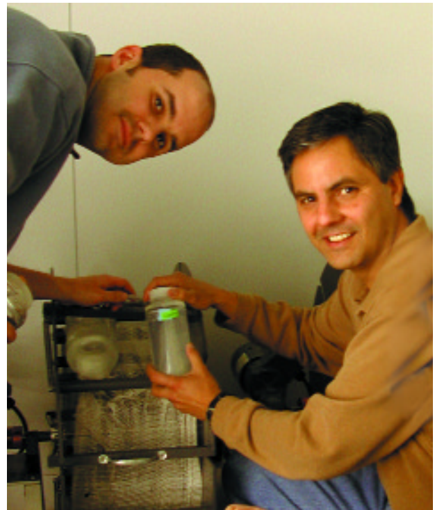
Hans Dam, right, and Sean Colin, left, put samples into a “plankton wheel”. Like a miniature ferris wheel, this equipment simulates the natural conditions in which plankton move with the flow of water.
