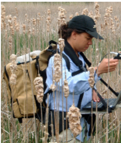
Dr. Marty Gilmore using a portable ASD spectrometer to collect spectra of a year-old cattail flower.
