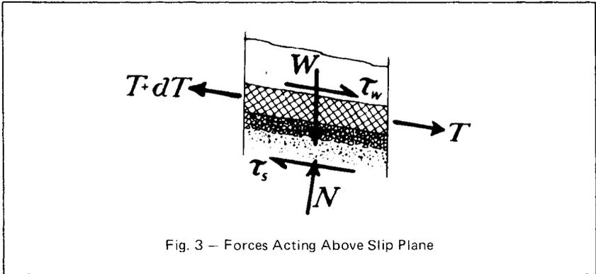
unit weight of water,  $\gamma$  the depth of flow, and  $S_0$  the slope of the water surface, energy gradient, and sauges. In practical cases, these slopes will not be identical and the flow will not be at a uniform depth. Estimating the important value of  $\tau_w$ , then, can be done conservatively by first computing the highest value of the velocity that can occur, then assuming that the shear is the same as it would be for uniform flow at that velocity, so that
