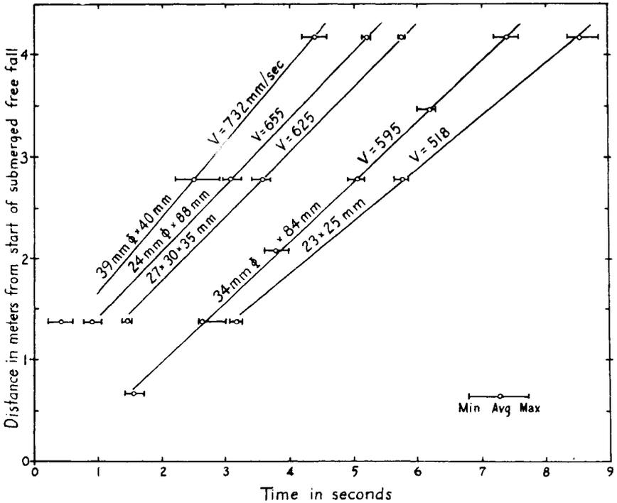
Fig. 2 DETERMINATION OF FALL VELOCITIES OF ROCK SAUSAGES
